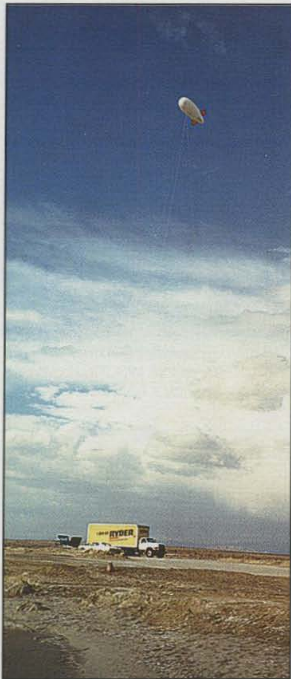
Photo A— The authors operate various 160 meter contests from the shore of the inland Salton Sea, using a rental truck to transport their equipment, including the aerostat (balloon) to support the antenna.
